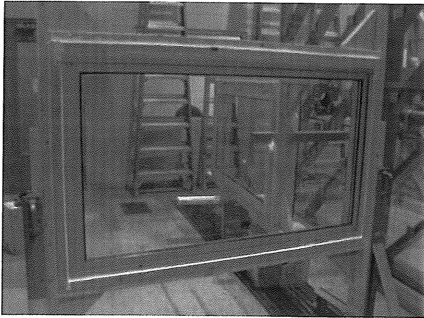
VW 3700 Photo No. 1 Project-Out Window
